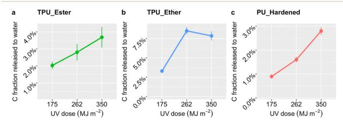
Fig. 2 Carbon mass fraction released from TPU\_Ester (a), TPU\_Ether (b), and PU\_Hardened (c) microplastics to the seawater as a function of cumulative UV dose in megajoule per square meter (MJ  $m^{-2}$ ). The dose values on the x-axis are plotted as factorial variables to improve data visualization. Data points and error bars represent the mean values and standard deviations, respectively, obtained from three replicate samples. Invisible error bars are smaller than the data point markers.
