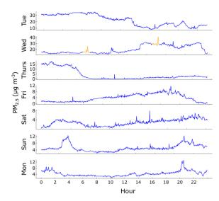
Fig. 9  $\sigma_{\Delta PM}$  filter applied to unit ccc9 for the first week in June 2021. Blue data points correspond to periods of low  $\sigma_{\Delta PM}$ , yellow data points correspond to periods of high  $\sigma_{\Delta PM}$
