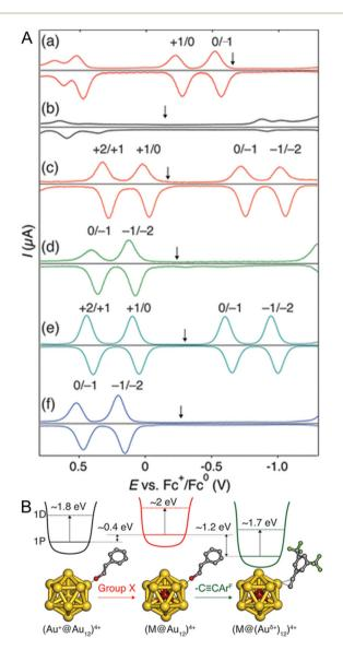
Fig. 8 (A) Differential pulse voltammograms of (a)  $[Au_{25}(PET)_{18}]^-$ , (b) M TBAPF<sub>6</sub> at room temperature. The down arrows indicate the corresponding open-circuit potentials. (B) Schematic energy diagram of  $M@Au_{12}$  superatoms protected by thiolate or alkynyl groups. Reproduced with permission from ref. 104. Copyright 2019, American Chemical Society.
