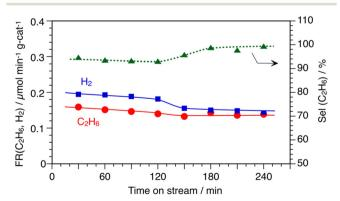
Fig. 1 Time courses of DCM reaction by  $In/SiO_2$  catalyst at 873 K.  $CH_4$ : 1 atm and 10 mL min<sup>-1</sup>, catalyst: 10 wt%  $In/SiO_2$ .
