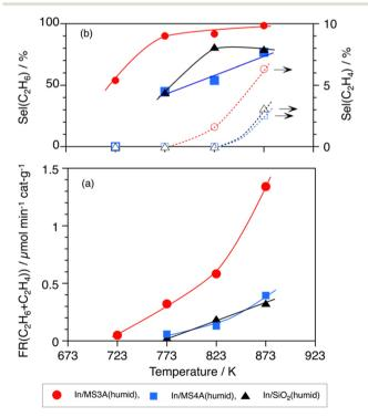
Fig. 4 Effects of reaction temperatures on the DCM reaction by 10 wt% In/MS3A(humid), 10 wt% In/MS4A(humid), and 10 wt% In/SiO<sub>2</sub>(humid) catalysts. (a) Formation rate of the sum of C<sub>2</sub>H<sub>6</sub> and C<sub>2</sub>H<sub>4</sub>; and (b) selectivity to  $C_2H_6$  and  $C_2H_4$ . Amount of catalyst: 100 mg,  $CH_4$ : 1 atm and 10 mL min<sup>-1</sup>
