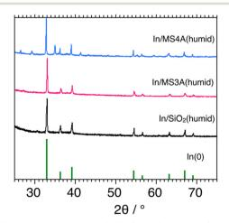
Fig. 5 XRD patterns of 10 wt% In/MS3A(humid), 10 wt% In/MS4A(humid), and 10 wt% In/SiO<sub>2</sub>(humid) flesh catalysts.
