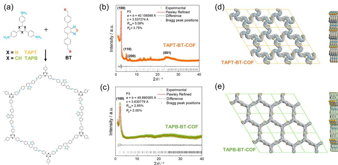
**Fig. 1** (a) Schematic overview of the synthesis of TAPT-BT-COF and TAPB-BT-COF. PXRD profile fits (Pawley method) of TAPT-BT-COF (b) and TAPB-BT-COF (c). Top view (left) and side view (right) of the AA packing mode of TAPT-BT-COF (d) and TAPB-BT-COF (e).
