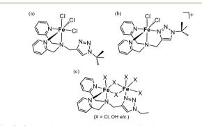
Fig. 2 Schematic drawings of the coordination structures of the iron(III) complexes. (a)  $[FeCl_3L']$  (ref. 18), (b)  $[FeCl_2L']^+$  (ref. 18), and (c) possible structures of the iron complex on the FeCl<sub>3</sub>-derived catalysts.
