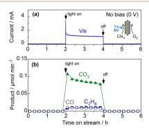
Fig. 9 PEC oxidation of CH<sub>4</sub> by the PEM-PEC reactor using the WO<sub>3</sub> photoanode and Pt/carbon catalyst: (a) the overall current at zero bias, and (b) the rate of products formation on the photoanode side under 453 nm light irradiation (6.8 mW cm<sup>-2</sup>).
