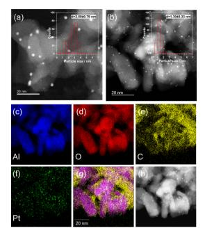
Fig. 2 HAADF-STEM images and particle size distribution of (a) fresh and (b) spent Pt(1)/Al<sub>2</sub>O<sub>3</sub>. EDX mapping images for (c) Al, (d) O, (e) C, (f) Pt, (g) overlay of (c-f), and (h) HAADF-STEM image of the spent catalyst. Spent catalyst: DCM was performed on Pt(1)/Al<sub>2</sub>O<sub>3</sub> for 5 h under CH<sub>4</sub>/H<sub>2</sub> (20/1).
