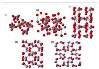
**Fig. 1** Structures of (a) trigonal BiPO<sub>4</sub>·(H<sub>2</sub>O)<sub>0.67</sub>, (b) monoclinic BiPO<sub>4</sub> ( $P_21/n$ ), and (c) monoclinic BiPO<sub>4</sub> ( $P_21/m$ ), (d) monoclinic  $\alpha$ -Bi<sub>2</sub>O<sub>3</sub>, and (e) tetragonal  $\beta$ -Bi<sub>2</sub>O<sub>3</sub>. Purple, gray, and red spheres represent Bi, P, and O atoms, respectively.
