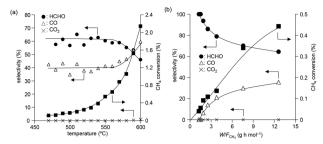
Fig. 4 (a) Product selectivity and CH<sub>4</sub> conversion as function of reaction temperature with O2 over BiPO4-DEG. Reaction conditions: BiPO<sub>4</sub>-DEG (100 mg),  $CH_4/O_2/N_2$  (2/2/6 sccm). (b) Effect of W/F<sub>CH4</sub> on product selectivity and CH<sub>4</sub> conversion. Reaction conditions: BiPO<sub>4</sub>-DEG (100 mg), CH<sub>4</sub>/O<sub>2</sub>/N<sub>2</sub> (38:8:54 molar ratio; total 7.8-78 sccm), reaction temperature (550 °C).
