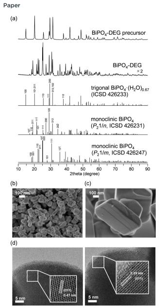
Fig. 2 (a) XRD patterns for BiPO<sub>4</sub>-DEG precursor, BiPO<sub>4</sub>-DEG, trigonal BiPO<sub>4</sub>·(H<sub>2</sub>O)<sub>0.67</sub> (ICSD 426233), monoclinic BiPO<sub>4</sub> (P<sub>2</sub>1/n, ICSD 426231), and monoclinic BiPO<sub>4</sub> (P<sub>2</sub>1/m, ICSD 426247). SEM images for (b) BiPO<sub>4</sub>-DEG and (c) BiPO<sub>4</sub>-HT. (d) TEM images for BiPO<sub>4</sub>-DEG.
