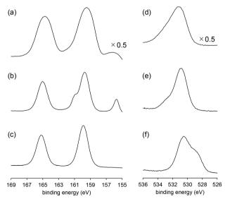
Fig. 7 XPS (a-c) Bi 4f and (d-f) O 1s spectra of BiPO<sub>4</sub>-DEG. (a and d) BiPO<sub>4</sub>-DEG at room temperature under evacuation, (b and e) BiPO<sub>4</sub>-DEG at 550 °C under evacuation, and (c and f) BiPO<sub>4</sub>-DEG at 550 °C under O<sub>2</sub> (0.1 mbar).
