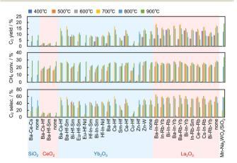
Fig. 5 Catalytic performance of the 28 predicted catalysts for the OCM reaction together with only supports and Mn-Na<sub>2</sub>WO<sub>4</sub>/SiO<sub>2</sub> for comparison.
