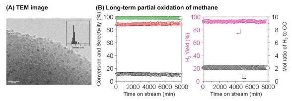
Fig. 18 (A) TEM image of 5 wt% Ni/MOR catalyst and (B) long-term partial oxidation of methane over the Ni/MOR catalyst. Reaction conditions:  $CH_4/O_2/Ar = 0.06/0.03/0.91$  atm;  $SV = 3.0 \times 10^4$  mL  $h^{-1}$   $g_{cat}^{-1}$ ; 973 K. Reproduced from ref. 77 with permission from Springer Nature, copyright 2020.
