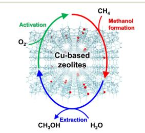
Fig. 8 Schematics of chemical looping process for partial oxidation of methane to methanol over Cu-based zeolites.
