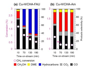
Fig. 14 Catalytic performance of (a) Cu-H/CHA-FAU and (b) Cu-H/ CHA-Am in the partial oxidation of methane. Reaction conditions: 100 mg catalyst;  $P_{CH_4}$ :  $P_{N_2O}$ :  $P_{H_2O}$ :  $P_{Ar}$  = 0.4:0.4:0.08: balance; total pressure 0.1 MPa; SV = 15 000 mL h<sup>-1</sup>  $g_{cat}^{-1}$ ;  $W/F = 3.7 g_{cat} h mol_{CH_4}^{-1}$ ; 623 K. Reprinted from ref. 63 with permission from Royal Society of Chemistry, copyright 2023.
