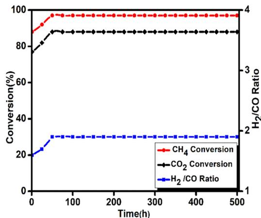
Fig. 8 Effect of time on stream for 5Ni-5Co-mod alumina at 850 °C with WHSV 10 L g<sup>-1</sup> h<sup>-1</sup> at atmospheric pressure. Prior to the activity study, the catalyst was reduced at 850 °C with 20% H<sub>2</sub>/N<sub>2</sub>.
