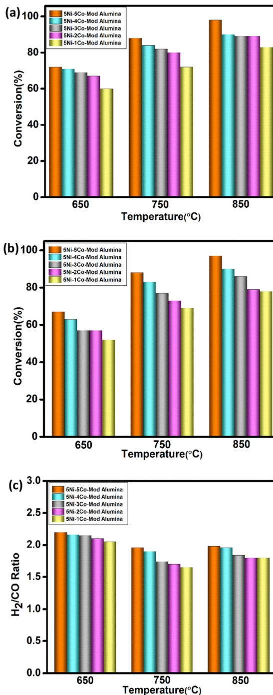
Fig. 5 Effect of temperature over the catalyst compositions at 10  $\text{L g}^{-1} \text{h}^{-1}$  WHSV and at atmospheric pressure (a)  $\text{CH}_4$  conversion (b)  $\text{CO}_2$  conversion (c)  $\text{H}_2/\text{CO}$  ratio. Prior to the activity study, the catalyst was reduced at 850 °C with 20%  $\text{H}_2/\text{N}_2$ .
