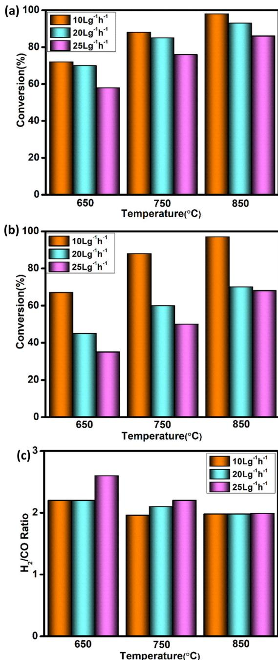
Fig. 6 Effect of space velocity and temperature on the catalytic activity under atmospheric pressure (a) CH<sub>4</sub> conversion (b) CO<sub>2</sub> conversion (c) H<sub>2</sub>/CO ratio of 5Ni-5Co-mod alumina. Prior to the activity study, the catalyst was reduced at 850 °C with 20% H<sub>2</sub>/N<sub>2</sub>.
