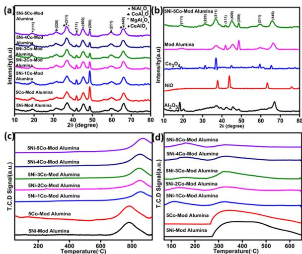
**Fig. 2** (a) and (b) XRD profile, (c) H<sub>2</sub>-TPR profile, and (d) CO<sub>2</sub>-TPD profile of the freshly synthesized catalysts.
