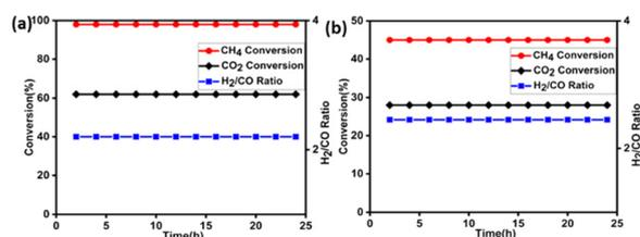
Fig. 7 Effect of time on stream on (a) 5Ni-mod alumina (b) 5Co-mod alumina at 850 °C with WHSV 10 L g<sup>-1</sup> h<sup>-1</sup> at atmospheric pressure. Prior to the activity study, the catalyst was reduced at 850 °C with 20% H<sub>2</sub>/N<sub>2</sub>.
