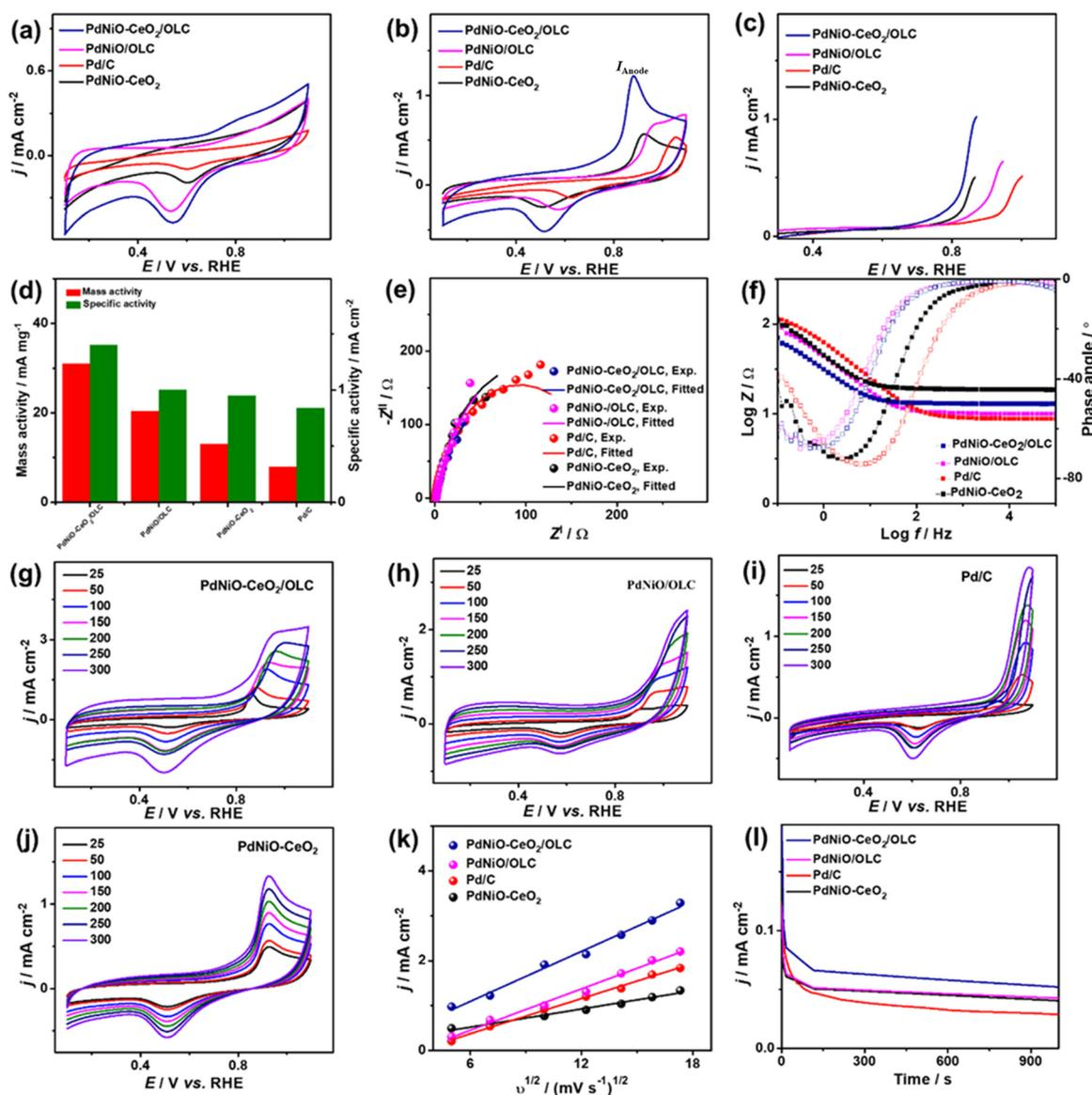
Fig. 5 CV profiles at 50 mV s<sup>-1</sup> in (a) N<sub>2</sub>-saturated NaHCO<sub>3</sub> (0.1 M) and (b) CO-saturated NaHCO<sub>3</sub> (0.1 M). (c) LSV at 50 mV s<sup>-1</sup>. (d) Mass/specific activities. (e) Nyquist plots. (f) Bode plots. (g–j) Scan rate studies. (k) Randles–Sevcik plots ( $I_{\text{Anode}}$  vs.  $\nu^{1/2}$ ) and (l) CA of PdNiO–CeO<sub>2</sub>/OLC, PdNiO/OLC, PdNiO–CeO<sub>2</sub>, and Pd/C in CO-saturated NaHCO<sub>3</sub> (0.1 M).
