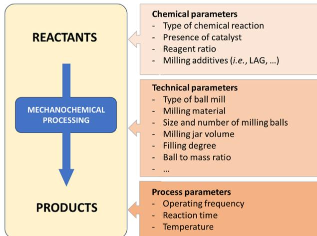
Fig. 2 Selected parameters to be taken into consideration during a ball-mill mechanochemical process.<sup>22</sup>
