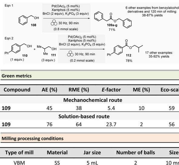
Scheme 25 Palladium-catalyzed oxidative self-esterification and cross-esterification by mechanochemistry.
