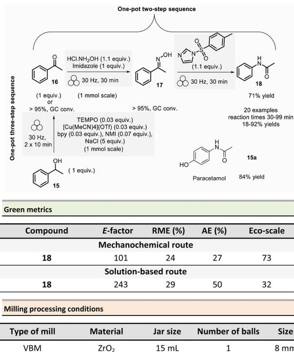
Scheme 4 *N*-Phenylacetamide preparation by mechanochemical Beckmann rearrangement.
