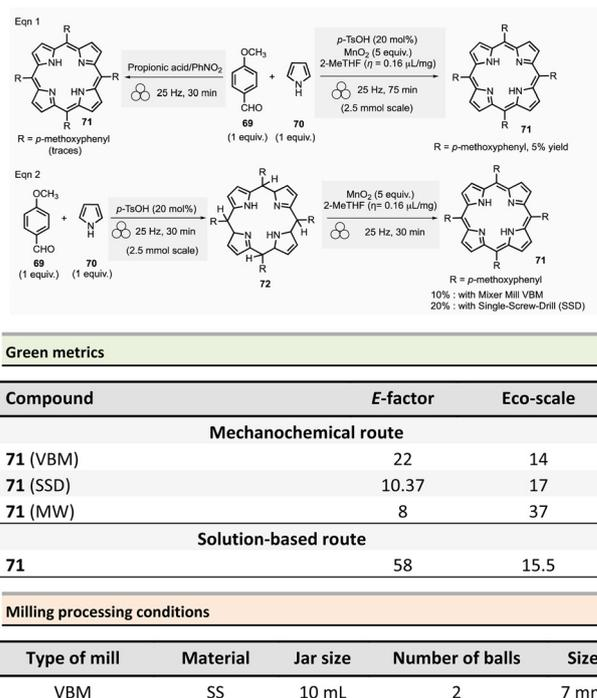
Scheme 16 One and two-step porphyrin syntheses by mechanochemistry.
