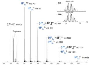
Fig. 2 ESI-MS spectrum of 10  $\mu$ M  $H^{W}_{Co}$  in  $H_{2}O$ , the 10+ to 5+ cage charge states are marked. Fragmentation products and cage species resulting from the loss of HBF<sub>4</sub> are also observed. The experimental vs. calculated m/z values for  $H^{W}_{Co}^{-10+}$  are shown in the inset.
