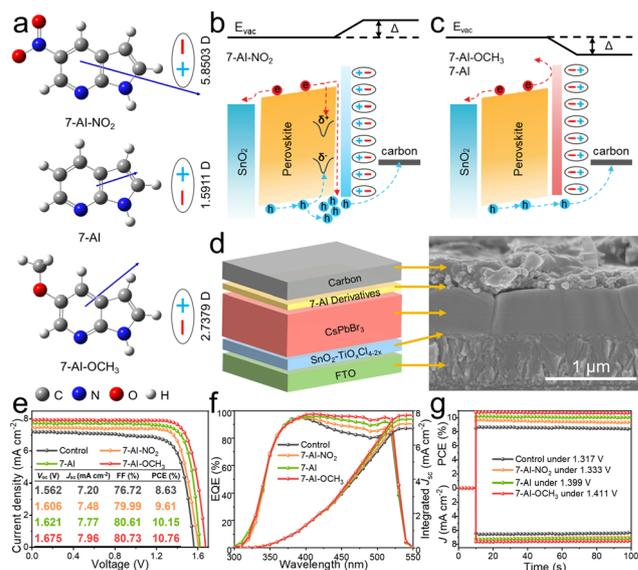
**Fig. 3** (a) Calculated dipole moment images of the three molecules. Schematic illustration of charge carrier collection and recombination in (b) 7-AI-NO<sub>2</sub>-based PSCs and (c) (AI or AI-OCH<sub>3</sub>)-based PSCs. (d) The architecture and cross-sectional SEM image of all-inorganic CsPbBr<sub>3</sub> PSCs. (e) The  $J$ - $V$  curves, (f) IPCE spectra, and (g) steady power output curves of various CsPbBr<sub>3</sub> PSCs.
