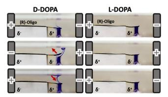
Fig. 8 Bipolar enantioselective valve operating with a Ppy actuator functionalized with (R)-oligo-BT<sub>2</sub>T<sub>4</sub> dipped in an aqueous 0.2 M LiClO<sub>4</sub> solution of 5 mM D-DOPA on the left and 5 mM L-DOPA on the right (Copyright © 2022, John Wiley and Sons).
