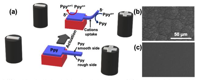
Fig. 4 (a) Schematic illustration of the electrochemical actuation mechanism of a Ppy polymer (blue) placed between two feeder electrodes, before and after applying an electric field. The Ppy film is intrinsically asymmetric, having a rough face (b) and a smooth one (c). (b and c) SEM micrographs at 50 μm of the two Ppy sides
