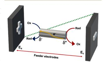
Fig. 3 General principle of bipolar electrochemistry.
