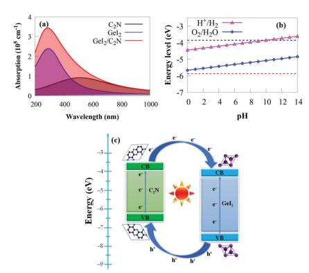
Fig. 6 (a) Calculated absorption spectra of the 2  $\times$  2 supercell of C<sub>2</sub>N, the 4  $\times$  4 supercell of Gel<sub>2</sub> and the Gel<sub>2</sub>/C<sub>2</sub>N vdW heterostructure. (b) The absolute energy bands for the conduction band minimum and valence band minimum of the  $Gel_2/C_2N$  vdW heterostructure with respect to pH (0-14). (c) Schematic diagram showing the transfer of photogenerated electrons and holes.
