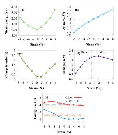
Fig. 7 (a) Strain energy, (b) binding energy, (c) charge transfer, (d) bandgap energies and (e) band edges of the Gel<sub>2</sub>/C<sub>2</sub>N vdW heterostructure under different biaxial strains. Green, orange, magenta, red and cyan dashed lines denote pH = 0, 3, 5, 7 and 9, respectively.
