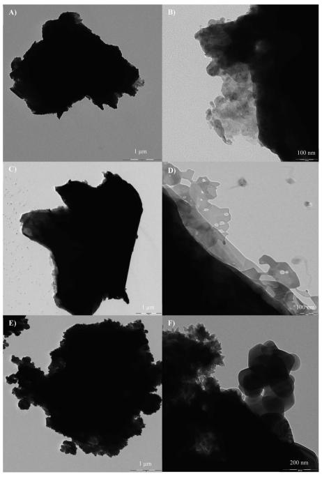
Fig. 4 TEM images of (A and B)  $Ti_3C_2$  MXene, (C and D)  $Ti_3C_2$  MXene aerogel, and (E and F)  $TiO_2/Ti_3C_2$  MXene aerogel composite.
