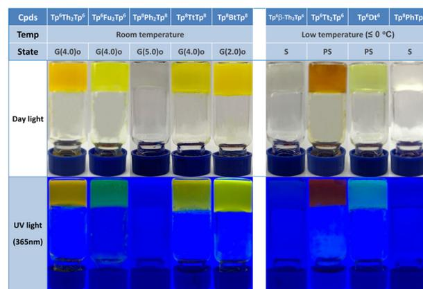
Fig. 10 Gels and frozen solutions of the dimers formed in cyclohexane on slow cooling, at room temperature and below 0 °C, in day light (top) and under UV irradiation (365 nm, bottom). G, S and PS indicate the state of the mixture corresponding to gel, solution and poor solution, respectively. The numbers in brackets correspond to the critical (minimum) gelation concentration (CGC/MGC) in mg mL<sup>-1</sup>; "o" indicates that the gel is opaque.
