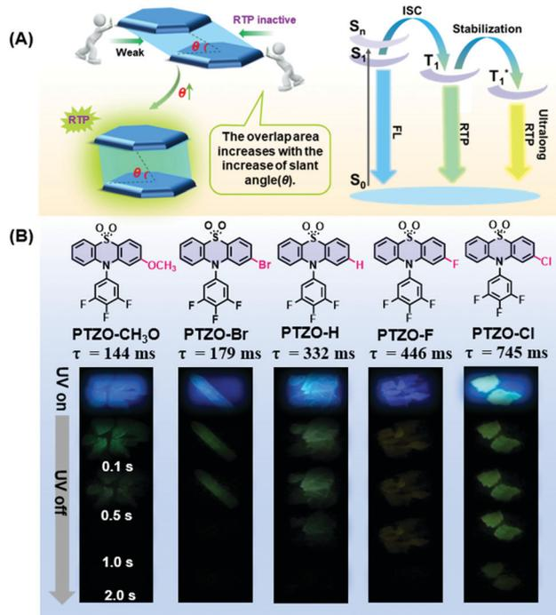
Fig. 1 (A) Strategy to promote the RTP performance. (B) Molecular structures of PTZO-CH<sub>3</sub>O, PTZO-Br, PTZO-H, PTZO-F and PTZO-Cl, and their corresponding photographs were taken before and after turning off the 365 nm UV irradiation under ambient conditions.
