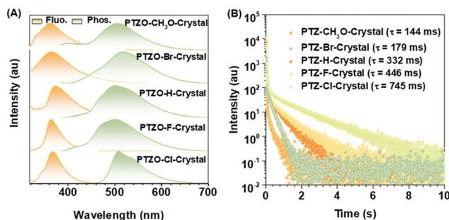
Fig. 2 (A) Normalized fluorescence (Orange line;  $\lambda_{ex}$  = 300 nm) and phosphorescence spectra (Green line;  $\lambda_{ex}$  = 365 nm) for PTZO-derivatives in the crystal state. (B) Room temperature phosphorescence decay curves of PTZO-derivatives in the crystal state.
