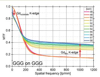
Fig. 4 Simulated MTFs for a 5 μm GGG:Eu SCF supported by 150 μm GGG substrate. X-ray energies from 48 to 58 keV. K-edge energy of Gd is 50.24 keV.
