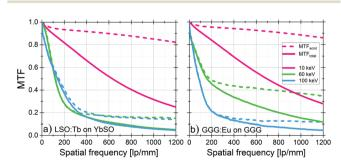
Fig. 5  $\,$  MTF  $_{tot}$  (solid lines) and MTF  $_{scint}$  (dashed lines) for 5  $\mu m$  films supported by 150  $\mu m$  substrates, evaluated for NA = 0.80 at different X-ray energies. The corresponding SCF, substrate and X-ray energies selected for the simulations are indicated in the figure
