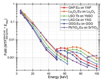
Fig. 6 The proposed figure of merit (FoM) calculated from the contrast in the MTF blurred by optics (NA = 0.40) at 500 lp mm<sup>-1</sup> and the energy deposited in the SCF. Values are extracted from simulations at X-ray energies from 5-100 keV for 5 μm SCFs supported by 150 μm substrates.
