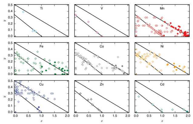
Fig. 4 The effect of M-site transition metal ions on the propensity for tilting. PBAs with composition  $A_xM[M'(CN)_6]_{1-y}\Box_y$  ( $\Box$  = vacancy) for various A, where filled (empty) symbols denote tilted (untilted) structures and the different panels refer to different M-site cations. The diagonal lines indicate compositions with a constant sum of the transition metal charges (+5 and +4).
