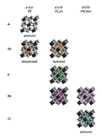
Fig. 3 Tilt patterns in Prussian blue analogues. The distribution of tilt patterns across PBAs with various A-site cations, where 'A' denotes the absence of A-site cations. The space group refers to the symmetry that the tilt gives rise to in the absence of further distortions. Tilts that (so far) are only known under pressure are indicated.
