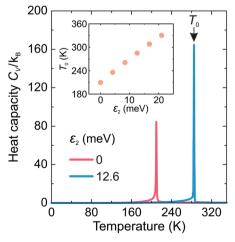
Fig. 4 Temperature dependence of the heat capacity of our model for  $\varepsilon_2$  = 0 and 12.6 meV. The anomalies mark the phase transition temperature  $T_0$ . The inset shows  $T_0$  vs.  $\varepsilon_2$  dependence. Other simulation parameters:
