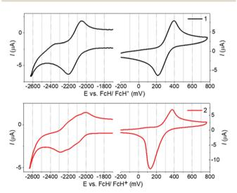
Fig. 3 Cyclic voltammograms for 1 and 2 measured in 0.1 M n-Bu<sub>4</sub>PF<sub>6</sub> in 1,2-dichlorobenzene as the supporting electrolyte. Scan rate = 100 mV s<sup>-1</sup>.
