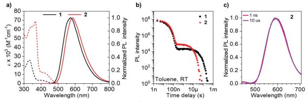
Fig. 4 (a) Extinction coefficient and steady state PL spectra ( $1 \times 10^{-5}$  M) of 1 and 2 in toluene; (b) PL decays of 1 and 2 in degassed toluene; (c) prompt and delayed time-resolved spectra for 2 in degassed toluene
