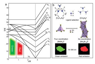
(a) Tanabe-Sugano (TS) energy diagram of 3d<sup>5</sup> electron orbital of Mn<sup>2+</sup>. (b) Modifying the coordination units of Mn<sup>2+</sup> by selecting different organic ligands to modulate the photoluminescence properties.
