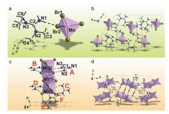
Fig. 1 Crystal asymmetric structure units of  $(C_5H_{14}N_3)_2MnBr_4$  (a) and (CH<sub>6</sub>N<sub>3</sub>)<sub>2</sub>MnBr<sub>4</sub> (c). The atoms in the asymmetric part of the unit cell  $(C_5H_{14}N_3)_2MnBr_4$  (b) and  $(CH_6N_3)_2MnBr_4$  (d) are labeled, the hydrogen bonds in which are presented as dashed lines. The independent [CH<sub>6</sub>N<sub>3</sub>]<sup>+</sup> cations in the Figure (c) are marked by bold labels A-E.
