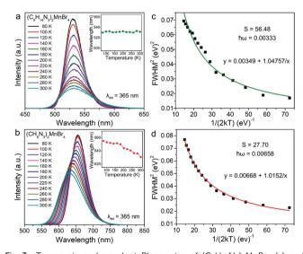
Fig. 3 Temperature-dependent PL spectra of (C<sub>5</sub>H<sub>14</sub>N<sub>3</sub>)<sub>2</sub>MnBr<sub>4</sub> (a) and  $(CH_6N_3)_2MnBr_4$  (b) under 365 nm excitation in the range from 80 to 300 K. Inset: the temperature-dependent emission peak. The FWHM fitting curve of  $(C_5H_{14}N_3)_2MnBr_4$  (c) and  $(CH_6N_3)_2MnBr_4$  (d) as a function of temperature via the eqn (4) to obtain the Huang-Phys factor S and maximum phonon energy  $\hbar\omega$
