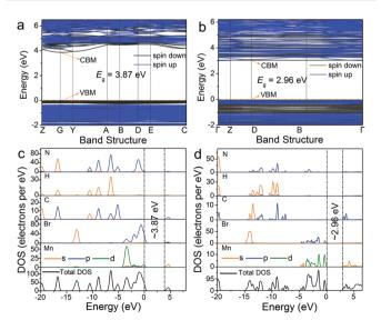
Fig. 5 Electronic energy band structures of (C<sub>5</sub>H<sub>14</sub>N<sub>3</sub>)<sub>2</sub>MnBr<sub>4</sub> (a) and (CH<sub>6</sub>N<sub>3</sub>)<sub>2</sub>MnBr<sub>4</sub> (b). The total and orbital projection of partial density of states of  $(C_5H_{14}N_3)_2MnBr_4$  (c) and  $(CH_6N_3)_2MnBr_4$  (d).
