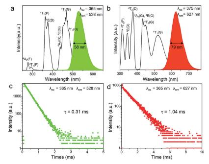
Fig. 2 The photoluminescence (PL) and photoluminescence excitation (PLE) spectra of  $(C_5H_{14}N_3)_2MnBr_4$  (a) and  $(CH_6N_3)_2MnBr_4$  (b) at room temperature (RT). Photoluminescence decay curves of  $(C_5H_{14}N_3)_2MnBr_4$  (c) and  $(CH_6N_3)_2MnBr_4$  (d) at RT under excitation at 365 nm, emission at 528/627 nm.
