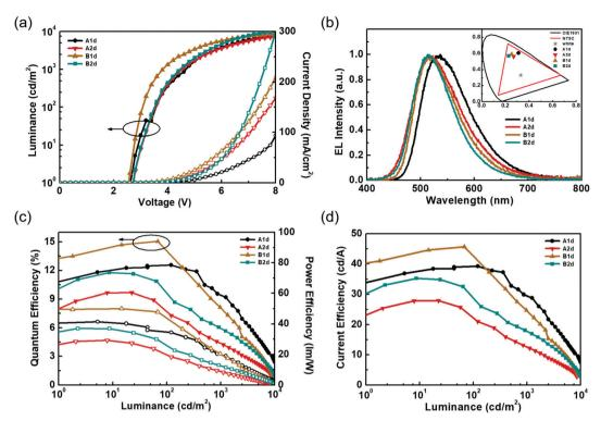
Fig. 5 EL characteristics of the OLED devices with different D/A combinations; (a) current density-voltage-luminance (J-V-L) curves, (b) normalized EL spectra and (inset) the CIE coordinates, (c) EQE and power efficiency (PE) as a function of luminance, and (d) current efficiency (CE)-luminance diagram.
