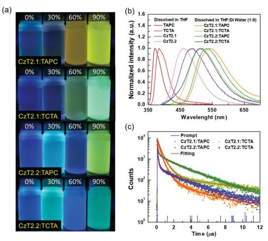
Fig. 2 (a) Photographs of four exciplex samples in THF with different water fractions under UV light illumination at room temperature, (b) normalized PL spectra of the D and A in THF and D: A (1:1) blends in THF with 90% water, and (c) the transient PL profiles of the D: A (1:1) blends in THF with 90% water.
