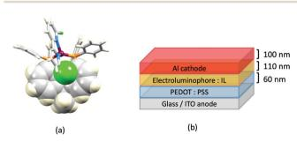
Fig. 10 (a) Structure of the cation in [Cu(xantphos)(6,6'-Cl<sub>2</sub>bpy)][PF<sub>6</sub>] (CSD refcode MEWXUK). (b) Architecture of LECs containing the CuiTMCs with halogen-substituted bpy ligands. IL = [EMIM][PF<sub>6</sub>] and CuiTMC: IL molar ratio = 4:1. LECs were driven using a pulsed current.
