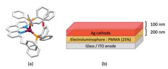
Fig. 4 (a) The structure of the  $[Cu(POP)(1)]^+$  cation in  $[Cu(POP)(1)][BF_4]$ (CSD refcode GIRJUN) showing the distorted tetrahedral Cu(i) environment and wide-bite angle (117.98(3)°) of POP (H atoms are omitted). The phen backbone is rigid (N-Cu-N = 80.86(10)°). (b) LEC architecture for a device containing [Cu(POP)(2)][BF<sub>4</sub>] as the electroluminophore.
