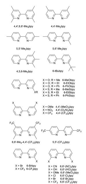
Scheme 4 Structures of derivatives of bpy used in [Cu(P^P)(N^N)]+ complexes. See also Scheme 2.
