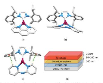
Fig. 24 Comparison of the structures of the [Cu(N^N)(NHC)]+ cations in (a) [Cu(phen)(42)][BF<sub>4</sub>] (CSD refcode SORNOE) and (b) [Cu(5-Mepy<sub>2</sub>NH)-(42)][PF<sub>6</sub>] (refcode SORPIA). (c) Intramolecular  $CH \cdots \pi$  interactions in [Cu(py<sub>2</sub>NH)(42)][PF<sub>6</sub>] (refcode SORPOG). (d) Architecture of the LECs containing Cu-iTMCs with NHC and py2NH-type N^N ligands; LECs were driven using a pulsed current.
