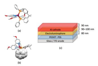
Fig. 9 (a) Structure of the cation in [Cu(xantphos)(4,4'-(MeO)<sub>2</sub>bpy)][BF<sub>4</sub>] (CSD refcode VANYOB), and (b) illustration of the  $\pi$ -stacking interaction between adjacent PPh2 units. H atoms are omitted for clarity. (c) Architecture of the LECs containing the Cu-iTMCs [Cu(xantphos)(4,4'-R2bpy)][BF4] with R = MeO, Me, H. LECs were driven using a pulsed current.
