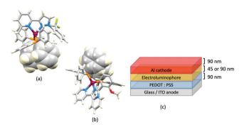
Fig. 16 Structures of the complex cations in (a)  $[Cu(POP)(8)][BF_4] \cdot EtOH$ (CSD refcode JUFNOP) and (b) [Cu(POP)(11)][PF<sub>6</sub>] showing Ph···arene  $\pi$ -stacking in the POP ligand (space-filling representation). (c) LEC architecture for testing with [Cu(POP)(11)][PF<sub>6</sub>] in the active layer; LECs were driven with a pulsed current.
