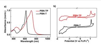
Fig. 3 (a) UV-vis-NIR absorption spectra and (b) cyclic voltammograms of PBN-TP and PBN-T in thin films.
