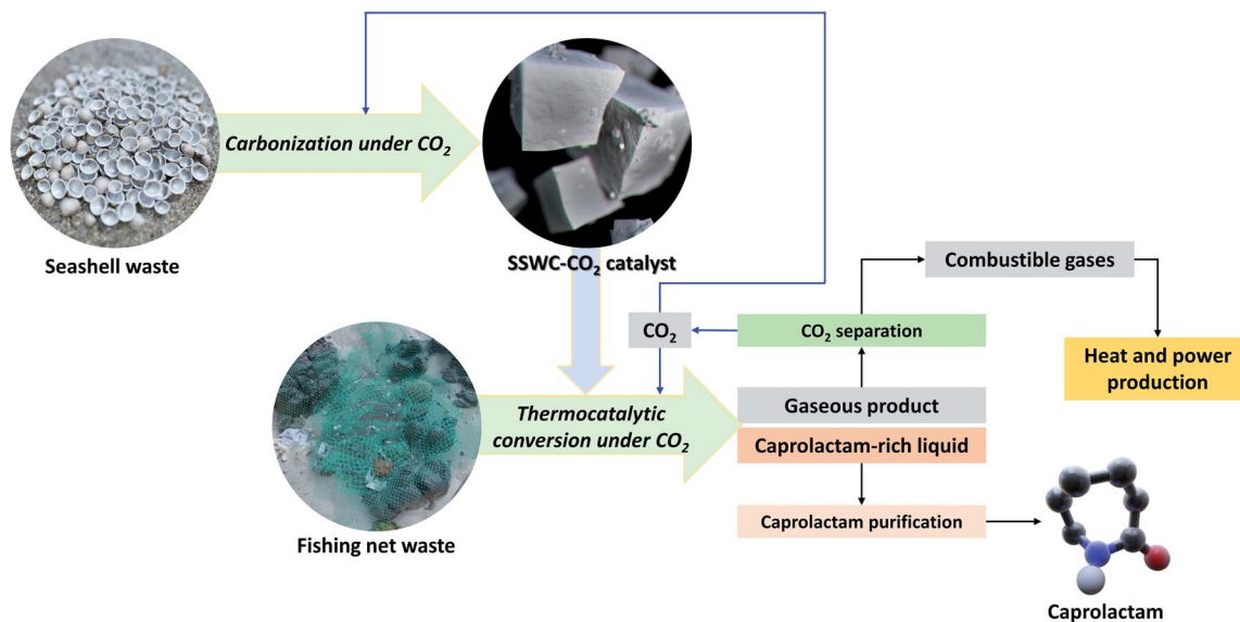
Fig. 10 Concept underpinning the thermocatalytic upcycling of marine waste (FNW and seashell waste) to monomer (caprolactam) under a CO 2 environment with the recycling of by-products.
