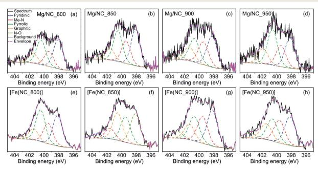
Deconvoluted XPS spectra in the N 1s region, for the (a)-(d) Mg/NC and (e)-(h) [Fe(N/C)] samples.
