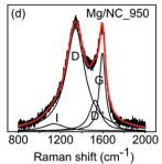
Fig. 3 Deconvoluted Raman spectra of the Mg/NC samples, pyrolyzed at different temperatures.
