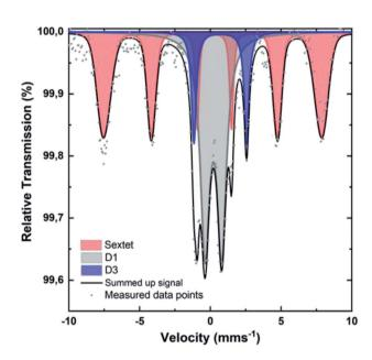
Fig. 6 Mössbauer spectrum of [Fe(N/C\_900)] obtained at 4.2 K.
