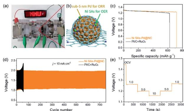
Fig. 6 (a) An LED bulb ( $\sim 5.0$  V) powered by three Zn–air batteries. (b) Schematic configuration of a Zn–air battery assembled with Ni SAs-Pd@NC. (c) Discharge curves at a constant current density of 5 mA cm<sup>-2</sup>. (d) The discharge and charge voltage profiles of Zn–air batteries with Ni SAs-Pd@NC at 10 mA cm<sup>-2</sup>. (e) Discharge profiles at different current densities (open-circuit voltage (OCV), 1.00, 5.00, and 10.00 mA cm<sup>-2</sup>, and recovery to OCV).
