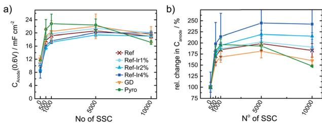
Fig. 8 (a) Change in capacitance and relative change in capacitance as a function of the number of SSC cycles applied to the catalysts. Values extracted from CV measurements in  $N_2$  saturated 0.1 M  $H_2SO_4$ .
