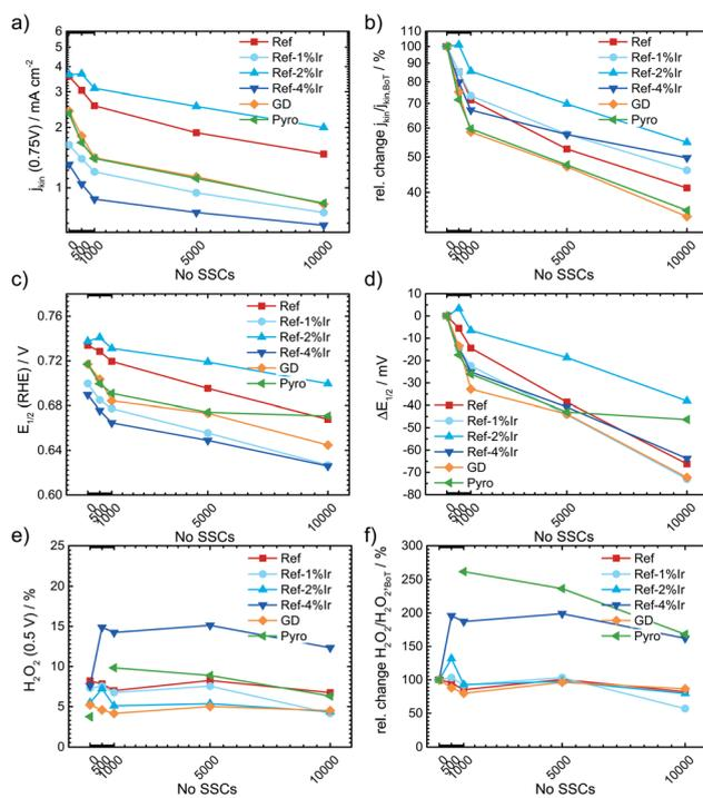
Fig. 9 Change in kinetic current density (a) absolute scale, (b) relative scale, half wave potential (c) absolute value, (d)  $\Delta E_{1/2}$  and hydrogen peroxide formation (e) absolute and (f) relative as a function of the number of SSCs.
