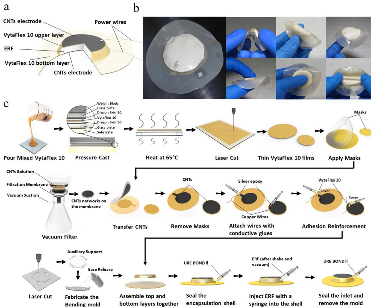
**Fig. 1** Design and manufacturing of the VSERF device. (a) Sandwiched configuration of the VSERF device with the CNT electrodes distributed in the very outer layers of the device and the ERF encapsulated in the chamber formed by two layers of VytaFlex 10 films. (b) Photographs show the characteristics of thin, soft, and stretchable VSERF, which will enable this device to be integrated with various systems. (c) Manufacturing processes of the VSERF.
