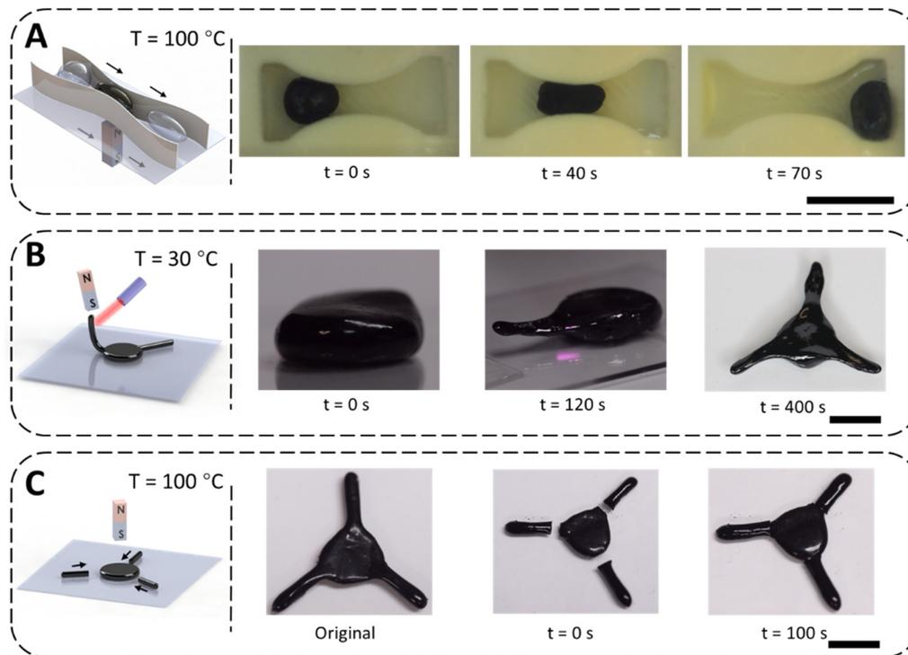
Fig. 4 Heat enabled flowability, remote shape morphing and self-healing of MV. (A) At an elevated temperature (100 °C), an MV sphere can pass through a narrow opening with an applied magnetic field. Scale bar, 1 cm. (B) An MV disk can transform into a soft gripper by applying local heating with a laser beam and a magnetic field by a permanent magnet. Scale bar, 1 cm. (C) Self-healing capability of the soft gripper after severe damage. Scale bar, 1 cm.
