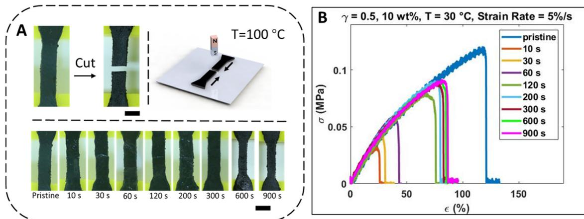
**Fig. 5** Magnetically assisted self-healing of MV. (A) MV strips were first cut into two parts at 30 °C. Then, assisted by the external magnetic field, the two broken parts were brought into contact and heated up at a temperature of 100 °C to trigger the dynamic bond exchange reaction. Specimens were healed for different time periods. Scale bar, 2 mm. (B) Tensile stress–strain relationship of self-healed MV strips with different healing times.
