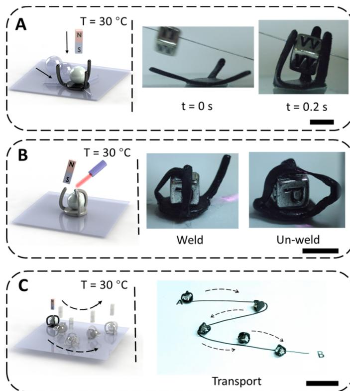
**Fig. 6** MV-based soft gripper. (A) The soft robotic gripper can catch a moving object through fast actuation. Scale bar, 1 cm. (B) Welding/un-welding of the gripper to secure/release the object. Scale bar, 1 cm. (C) With an externally applied magnetic field, the soft robotic gripper can carry the object and move along a planned path. Scale bar, 5 cm.
