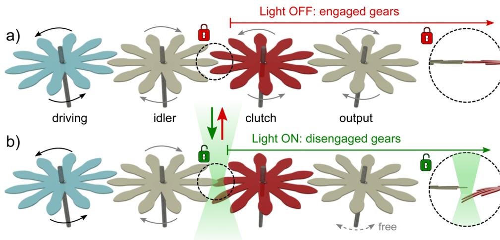
Fig. 1 Concept of the powertrain transmission consisting in a gear train with active gears. The driving gear powers the gear train via onboard chemical motors. The clutch gear, fabricated from PLCNs, is photothermally activated to (a) engage and (b) disengage from the gear train.
