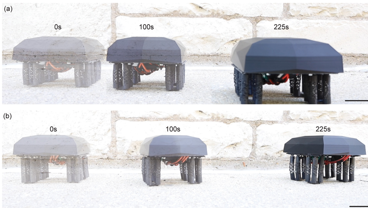
Fig. 6 Untethered soft robotic quadrupeds. Untethered HSA-based soft robots constructed with the (a) 0.5 \times legs and (b) stilted 0.5 \times legs are shown walking on a concrete sidewalk. Overlays of the quadrupeds are shown at 0 s, 100 s, and 225 s of the walking sequence. Stills are taken from Movie S4 in the ESI.† Scale bars are 50 mm.
