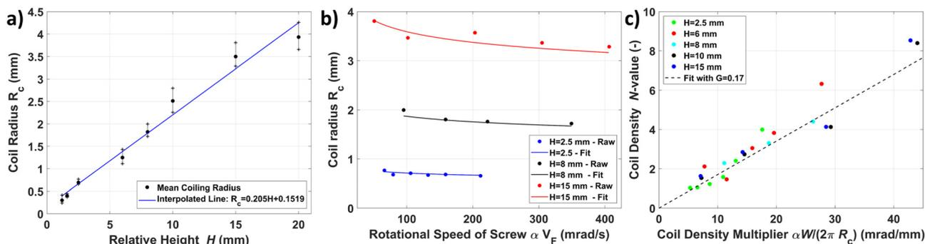
Fig. 3 (a and b) Coil radius versus height  $H$  (a) and (b) rotational speed of screw ( $\alpha V_F$ ), and (c) the coil density ( $N$ -value) versus coil density multiplier ( $\alpha W/(2\pi R_c)$ ) used to estimate  $G$  (see eqn (3)).
