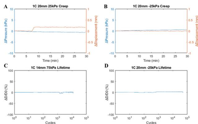
Fig. 4 Actuator Creep and Lifetime. (A) 1C 20 mm held at 25 kPa showing pressure and displacement creep. (B) 1C 20 mm held at  $-25$  kPa showing creep. (C) 1C 14 mm showing stroke lifetime at cycles of 75 kPa. (D) 1C 20 mm showing stroke lifetime at cycles of  $-25$  kPa.
