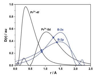
Fig. 3 Atomic valence-orbital radial-densities  $D(r) = r^2 R(r)^2$  of 4f/5d orbitals (black lines) of  $Pr^{3+}$  ion with  $4f^2$  configuration and of 2s/2p orbitals (blue lines) of B atom lying at 2.3 Å (from PBE density functional calculations).
