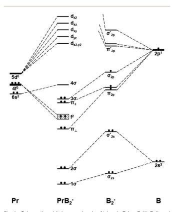
Fig. 4 Schematic orbital energy levels of triangle Pr( $\eta_2$ -B<sub>2</sub>)<sup>-</sup>, B<sub>2</sub><sup>-</sup>, and Pr. The symbol  $\pi_{\parallel}$  and  $\pi_{\perp}$  denotes the in-plane and out-of-plane  $\pi$  MOs, and their respective orbital interaction with Pr  $5d_{x^2-y^2}$  and  $5d_{xz}$  orbitals are shown in Scheme 1.
