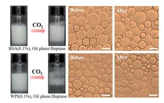
Fig. 3 CO<sub>2</sub>/N<sub>2</sub>-responsive behavior of emulsions stabilized using different types of proteins. Scale bar: 100 µm.
