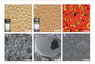
Fig. 1  $CO_2/N_2$ -switchable emulsions stabilized with 0.1 wt% NaCas. Optical micrographs and visual appearance of the emulsions using n-heptane as the oil phase after storage for 0 h (a) and 80 h (b). CLSM image (c) and cryo-SEM image (d–f) of the emulsions with n-heptane as the oil phase. Scale bar: (a–d) 100  $\mu$ m, (e) 30  $\mu$ m, and (f) 500 nm.
