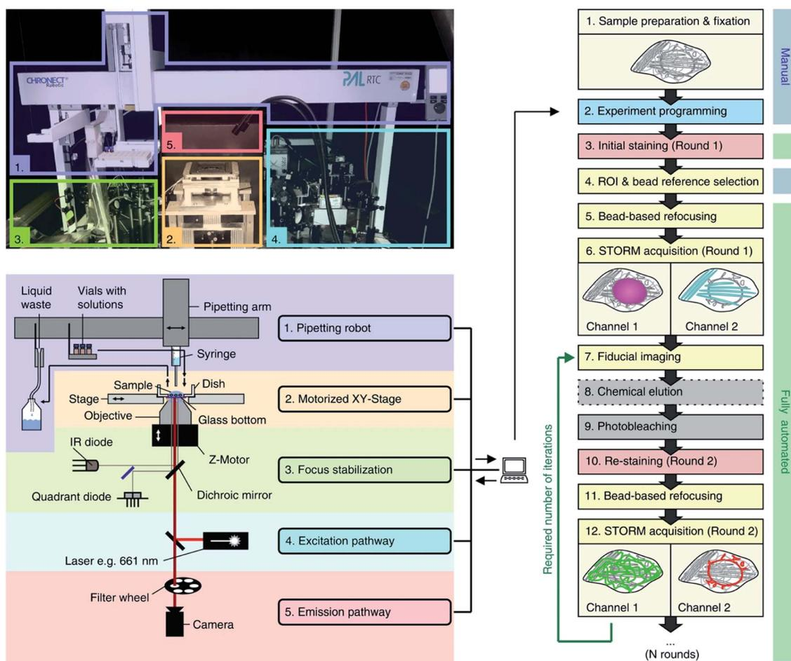
Fig. 5 Automated maS<sup>3</sup>TORM setup and workflow indicating photographic (upper left panel), and schematic outlines (lower left panel) and experimental details for an automated multiplex system (right panel). Reused with permission from ref. 115.
