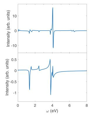
Fig. 8 CD signals eqn (9) of polariton in the chiral cavity with  $\delta = 0$ , g = $1.028 \times 10^{-1} \, \text{V Å}^{-1}$  (or  $0.002 \, \text{a.u.}$ ) (top), and no cavity (bottom). The CD measurement follows a circularly polarized pump pulse in both polariton and bare molecule.
