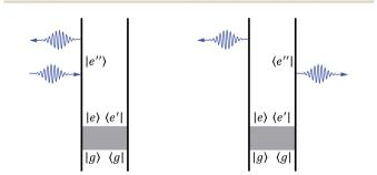
Fig. 2 Ladder diagrams of the circular dichroism signal. The left and right diagrams correspond to first and second term in eqn (9) respectively. The gray zone is the pump pulse with either a linearly polarized pulse or circularly polarized pulse. After the pump pulse, the polariton is excited and described by density matrix  $\rho_{ee'}$ . A CD measurement is done with circularly polarized pump pulse at a later time.
