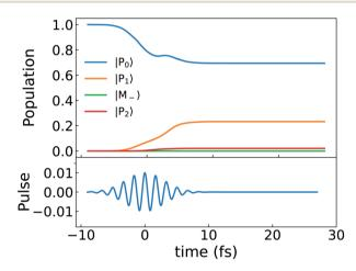
Fig. 6 Top: population dynamics (eqn (8)) of the polariton states for a Mg-porphyrin in the chiral cavity excited by a circularly polarized pulse. Bottom: y component of the electric field of the pump pulse.
