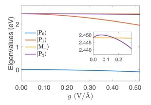
Fig. 3 Polariton energy variation with g for detuning  $\delta=0$ . The splitting of  $|P_1\rangle$  and  $|P_2\rangle$  increase with g. The energy of  $|P_2\rangle$  is lower than  $|M_-\rangle$  for g>0.16 V Å $^{-1}$ .
