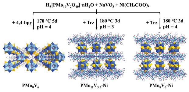
Fig. 1 Illustration of the PMoV-based hybrid materials preparation process (color code: C gray, N drak blue, O red, P pink, Mo blue, V yellow, Ni indigo, Mo/V light blue).
