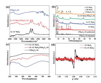
Fig. 3 (a) FT-IR spectra, (b) XRD patterns, and (c) UV-vis diffuse reflectance spectra of Sv-1T MoS<sub>2</sub>, PMo<sub>8</sub>V<sub>6</sub>-Ni, and Sv-1T MoS<sub>2</sub>/PMo<sub>8</sub>V<sub>6</sub>-Ni composite-materials, and (d) EPR spectra of 1T  $MoS_2$  and Sv-1T  $MoS_2$ .
