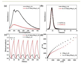
Fig. 6 (a) Steady PL spectra, (b) time-resolved PL spectra, (c) photocurrent responses, and (d) EIS Nyquist plots of PMo<sub>8</sub>V<sub>6</sub>-Ni and Sv-1T MoS<sub>2</sub>/PMo<sub>8</sub>V<sub>6</sub>-Ni.
