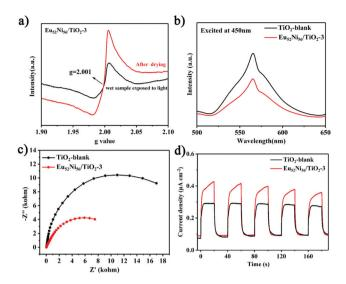
Fig. 4 (a) EPR spectra of wet  $Eu_{52}Ni_{56}/TiO_2$ -3 after light irradiation and after drying at 110 K. (b) Photoluminescence spectra of TiO<sub>2</sub>-blank and Eu<sub>52</sub>Ni<sub>56</sub>/TiO<sub>2</sub>-3 with excitation at 450 nm. (c) Electrochemical impedance spectroscopy of TiO<sub>2</sub>-blank and Eu<sub>52</sub>Ni<sub>56</sub>/TiO<sub>2</sub>-3. (d) Transient photocurrent response of TiO2-blank and Eu52Ni56/TiO2-3 under simulated irradiation and off.
