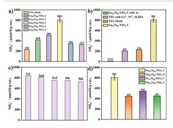
Fig. 3 (a) N<sub>2</sub> reduction activities of TiO<sub>2</sub>-blank and Eu<sub>52</sub>Ni<sub>56</sub>/TiO<sub>2</sub>-1, 2, 3, 4, 5. (b) Controlled experiments with TiO<sub>2</sub>-blank and Eu<sub>52</sub>Ni<sub>56</sub>/TiO<sub>2</sub>-3. (c) Five catalytic cycles of Eu<sub>52</sub>Ni<sub>56</sub>/TiO<sub>2</sub>-3. (d) N<sub>2</sub> reduction activities of  $Eu_{52}Ni_{56}/TiO_2-3$ ,  $Gd_{52}Ni_{56}/TiO_2-3$ ,  $Pr_{52}Ni_{56}/TiO_2-3$ , and  $Nd_{52}Ni_{56}/TiO_2-3$  $TiO_2-3$ .
