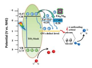
Fig. 5 Charge separation and transfer in the Eu<sub>52</sub>Ni<sub>56</sub>/TiO<sub>2</sub>-3 composite under light irradiation. VB: valence band; CB: conduction band.
