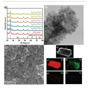
Fig. 1 (a) PXRD patterns of  $TiO_2$ -blank and  $Eu_{52}Ni_{56}/TiO_2$ -1, 2, 3, 4, 5. (b) TEM profile of  $Eu_{52}Ni_{56}/TiO_2-3$ . (c) SEM profile of  $Eu_{52}Ni_{56}/TiO_2-3$ . (d-h) Selected area SEM profile of Eu<sub>52</sub>Ni<sub>56</sub>/TiO<sub>2</sub>-3, and corresponding EDX elemental mappings of Ti, O, Eu, and Ni.
