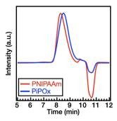
Fig. 2 GPC traces obtained for PNIPAAm (red line) and PiPOx (blue line) in DMF containing 10 mM LiBr.
