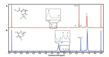
Fig. 1 <sup>1</sup>H NMR spectra of (a) PNIPAAm and (b) PiPOx after purification in CDCI-
