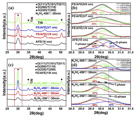
Fig. 4 (a) GIXRD patterns and (b) de-convolution of the diffraction peak of O (111)/T (101)/T (011) for the single AFE film and different FE/AFE stacks on the TiN film after annealing at 450 °C for 30 min; (c) GIXRD patterns and (d) de-convolution of the peak of O (111)/T (101)/T (011) for the FE (1 nm)/AFE (9 nm) stack on the TiN film after annealing at different temperatures for 30 min.
