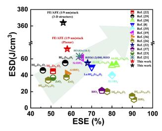
Fig. 9 Comparison of the achievable ESD and the ESE between our FE/AFE stack capacitors and other HfO<sub>2</sub>/ZrO<sub>2</sub>-based single AFE capacitors.
