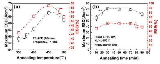
Fig. 3 The maximum ESD and corresponding ESE of the capacitor with the FE (1 nm)/AFE (9 nm) stack: (a) at different annealing temperatures for 30 min; (b) at 450 °C for different annealing times. Ten devices are measured for each sample.
