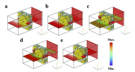
Fig. 4 Investigation on the electric field incident on and passing through the metasurface with different sets of resistance parameters corresponding to Fig. 3: (a)  $R_1 = 4.2 \ \Omega$ ;  $R_2 = \infty$ . (b)  $R_1 = 250 \ \Omega$ ;  $R_2 = \infty$ . (c)  $R_1 = \infty$ ;  $R_2 = \infty$ . (d)  $R_1 = \infty$ ;  $R_2 = 250 \ \Omega$ . (e)  $R_1 = \infty$ ;  $R_2 = 4.2 \ \Omega$ .
