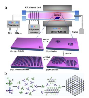
Fig. 4 Synthesis of NG by (a) the CVD method and (b) the WRC reaction. (a–c) Reprinted with permission from ref. 65 and 72, 2011 and 2015 copyright© American Chemical Society, respectively.
