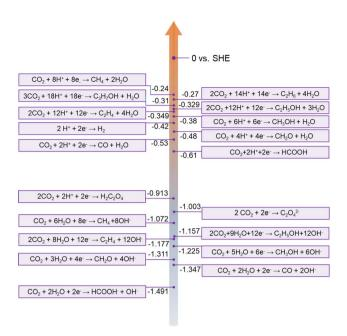
Fig. 7 CO<sub>2</sub>RR at different standard potentials in aqueous solution at pH = 7.0, 1.0 atm, and 25°C. Reprinted with permission from ref. 26, copyright© 2019 The Royal Society of Chemistry.
