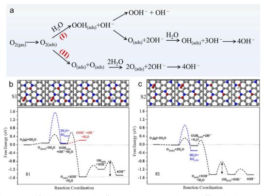
Fig. 5 (a) ORR pathways on NG in alkaline solution, where (I) presents an associative mechanism and (II) is a dissociative mechanism. (b) Free energy diagram for  $O_2$  reduction on  $S_1$  and  $S_2$  under the conditions of 0.04 V and pH = 14. (c) Intermediate structures of the associative mechanism on  $S_1$  and  $S_2$ . The gray, blue, red, and white spheres represent C, N, O, and H atoms, respectively. Reprinted with permission from ref. 80, Copyright©2012 Elsevier Inc.
