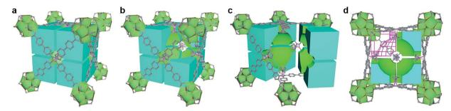
Fig. 12 Structural illustration of UPC-612 with cage filling. (a) Cubic cage filling of a basic unit in UPC-612; (b) space division of cubic cage; (c) internal space allocation of UPC-612 after partition; (d) cubic cage filling profile and a sphere like force surface. Reproduced from ref. 77 with permission, copyright John Wiley and Sons, 2021.
