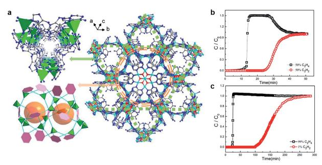
Fig. 6 (a) The channel and cavities in the 3D structure of NbU-1. (b) and (c) Breakthrough experiment for the mixture of  $C_2H_2$  and  $C_2H_4$  (50 : 50, 1 : 99, respectively). From the mixture of  $C_2H_2$  and  $C_2H_3$  and  $C_2H_4$  (50 : 50, 1 : 99, respectively).
