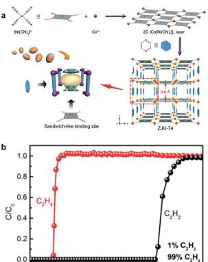
Fig. 8 (a) The construction process of ZJU-74a, 3D framework, and sandwich-like binding sites. (b) Experimental column breakthrough curves for a 1/99  $C_2H_2/C_2H_4$  mixture at 298 K and 1 bar.<sup>68</sup> Reproduced from ref. 68 with permission, copyright John Wiley and Sons, 2020.
